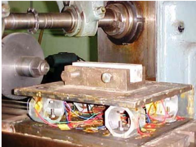
Milling force measurement – strain gauge octagonal ring setup
