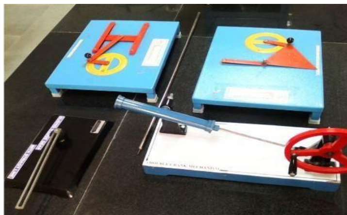
Prototypes of Inversions of Slider Crank Mechanism
