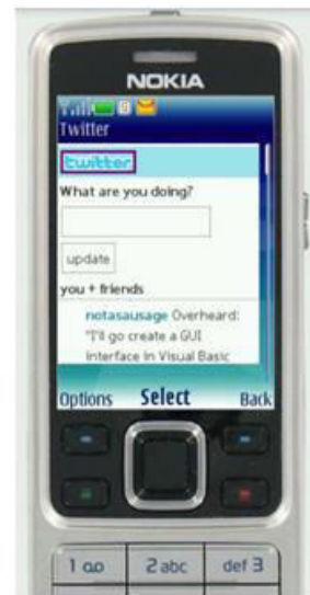
Figure 4.23. Example layout of a scroll-based application, where the user had to press the D-pad past each link to scroll the page
